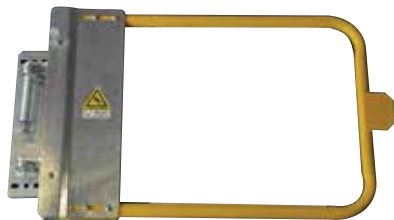
NORTH AMERICAN GATE 30" - POWDER COATED - SGNA030PC Spring Loaded, self-closing safety gate for North America. Each model can be adjusted on site for an additional 3" without need for cutting or welding. Complete with fixing pack. Powder Coated USA - AAMA 2603-2605. Material : Galvanised steel to ASTM A53. Net weight : 18.3kg (40lb 5oz).
