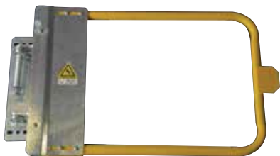
NORTH AMERICAN GATE 24" - POWDER COATED - SGNA024PC Spring Loaded, self-closing safety gate for North America. Each model can be adjusted on site for an additional 3" without need for cutting or welding. Complete with fixing pack. Powder Coated USA - AAMA 2603-2605. Material : Galvanised steel to ASTM A53. Net weight : 17.5kg (38lb 10oz).
