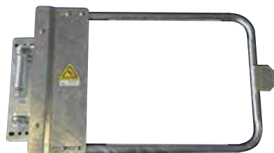
NORTH AMERICAN GATE 30" - GALVANISED - SGNA030GV Spring Loaded, 30" self-closing safety gate for North America. Each model can be adjusted on site for an additional 3" without need for cutting or welding. Complete with fixing pack. Material : Galvanised steel to ASTM A53. Net weight : 18.3kg (40lb 5oz).
