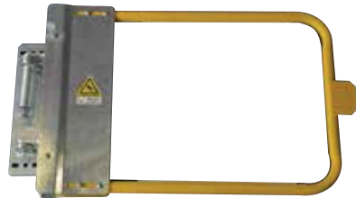
NORTH AMERICAN GATE 36" - POWDER COATED - SGNA036PC Spring Loaded, self-closing safety gate for North America. Each model can be adjusted on site for an additional 3" without need for cutting or welding. Complete with fixing pack. Powder Coated USA - AAMA 2603-2605. Material : Galvanised steel to ASTM A53. Net weight : 19kg (41lb 14oz).
