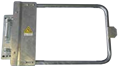
NORTH AMERICAN GATE 24" - GALVANISED - SGNA024GV Spring Loaded, self-closing safety gate for North America. Each model can be adjusted on site for an additional 3" without need for cutting or welding. Complete with fixing pack. Material : Galvanised steel to ASTM A53. Net weight : 17.5kg (38lb 10oz).
